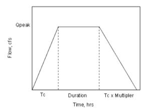
Qpeak is determined from the rational method (see definition for "Rational Method").
