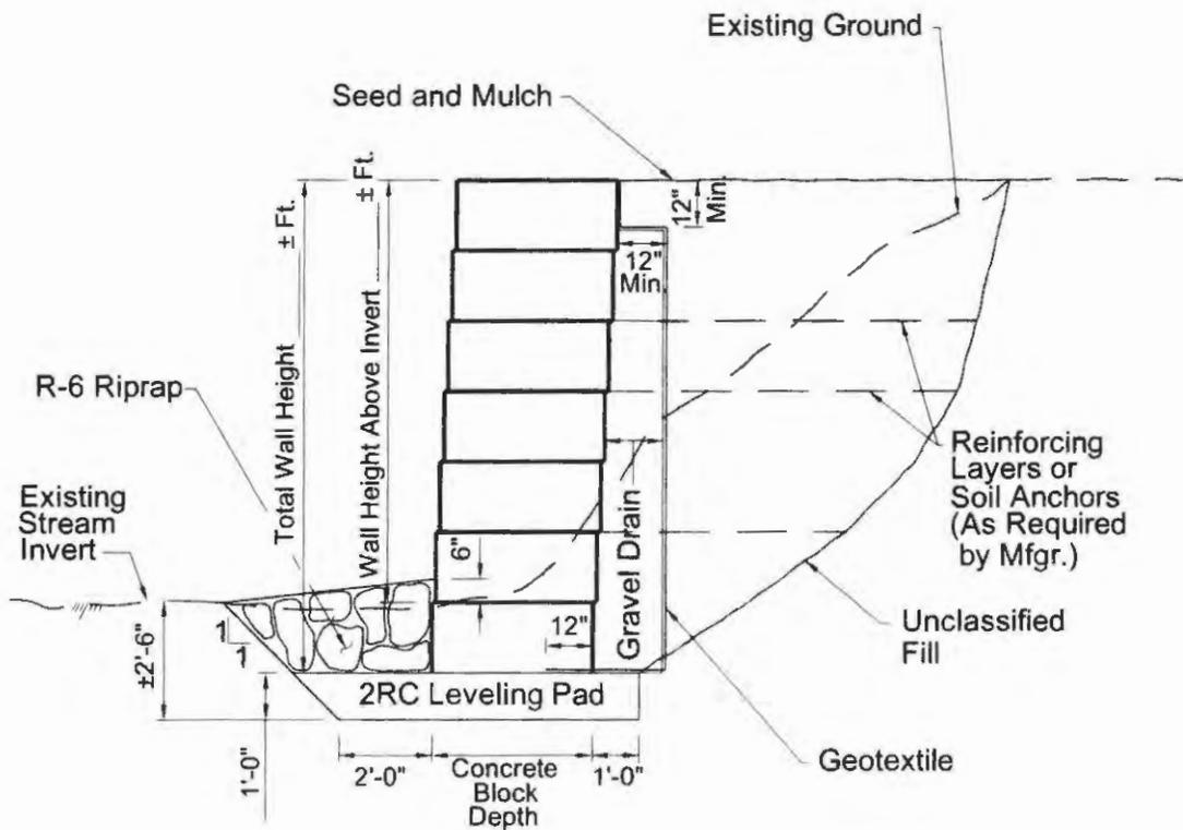
**PRECAST CONCRETE MODULAR BLOCK WALL (PCMBW) DETAIL**
